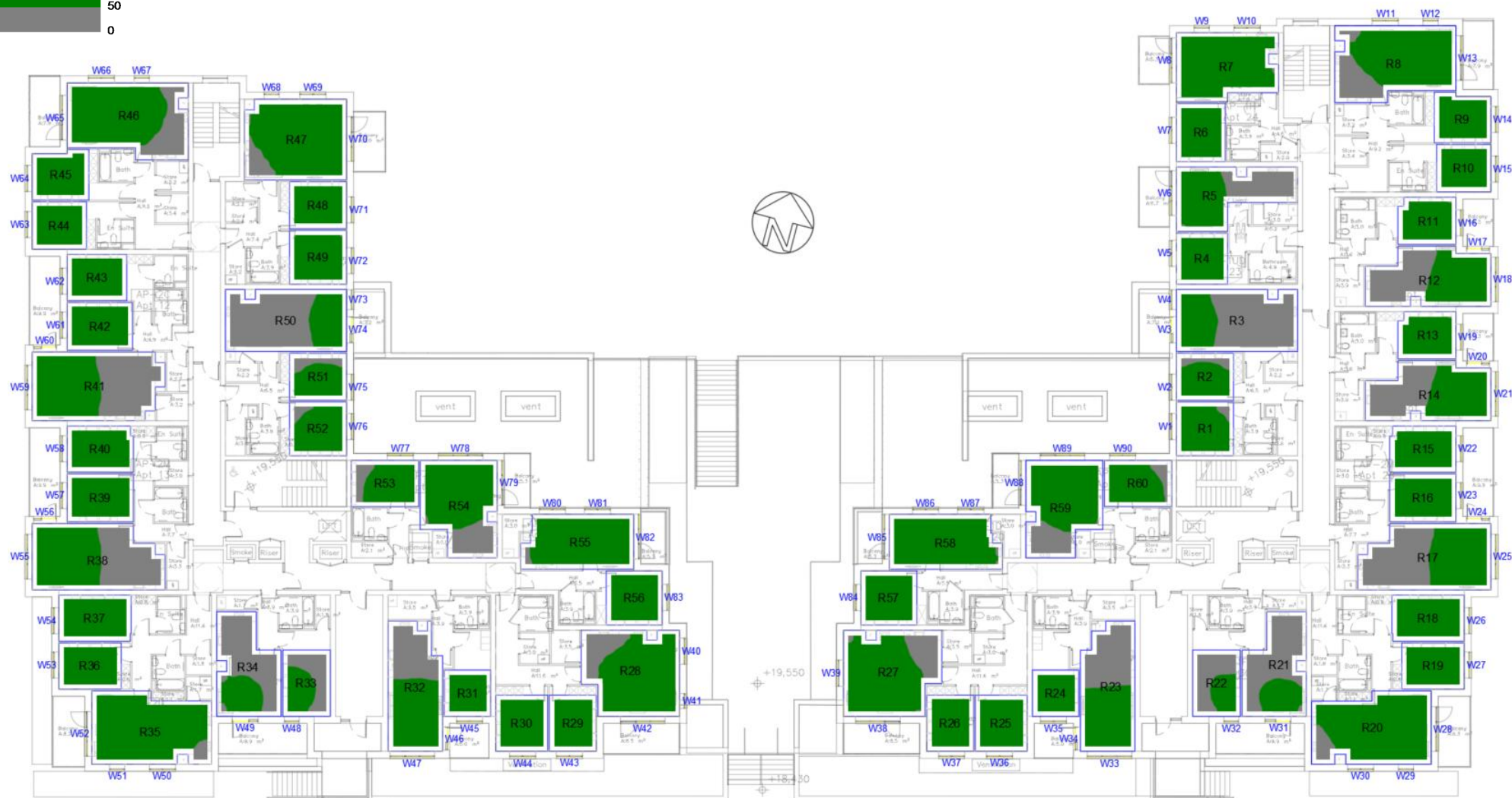
Figure 20: Resi. Apartment Ground Floor sDA Contours
