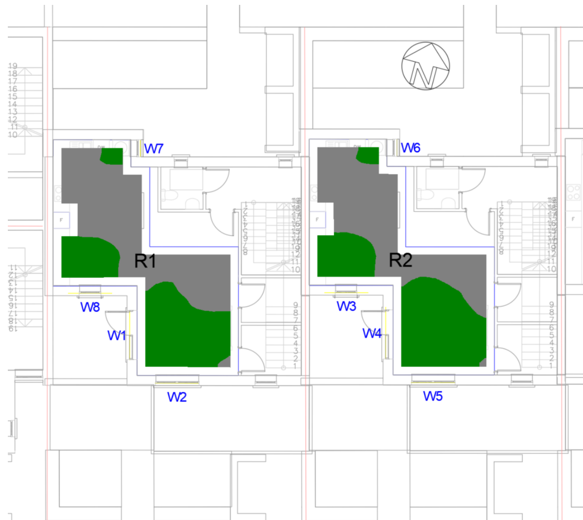
Figure 28: DP-03-04 First Floor sDA Contours
