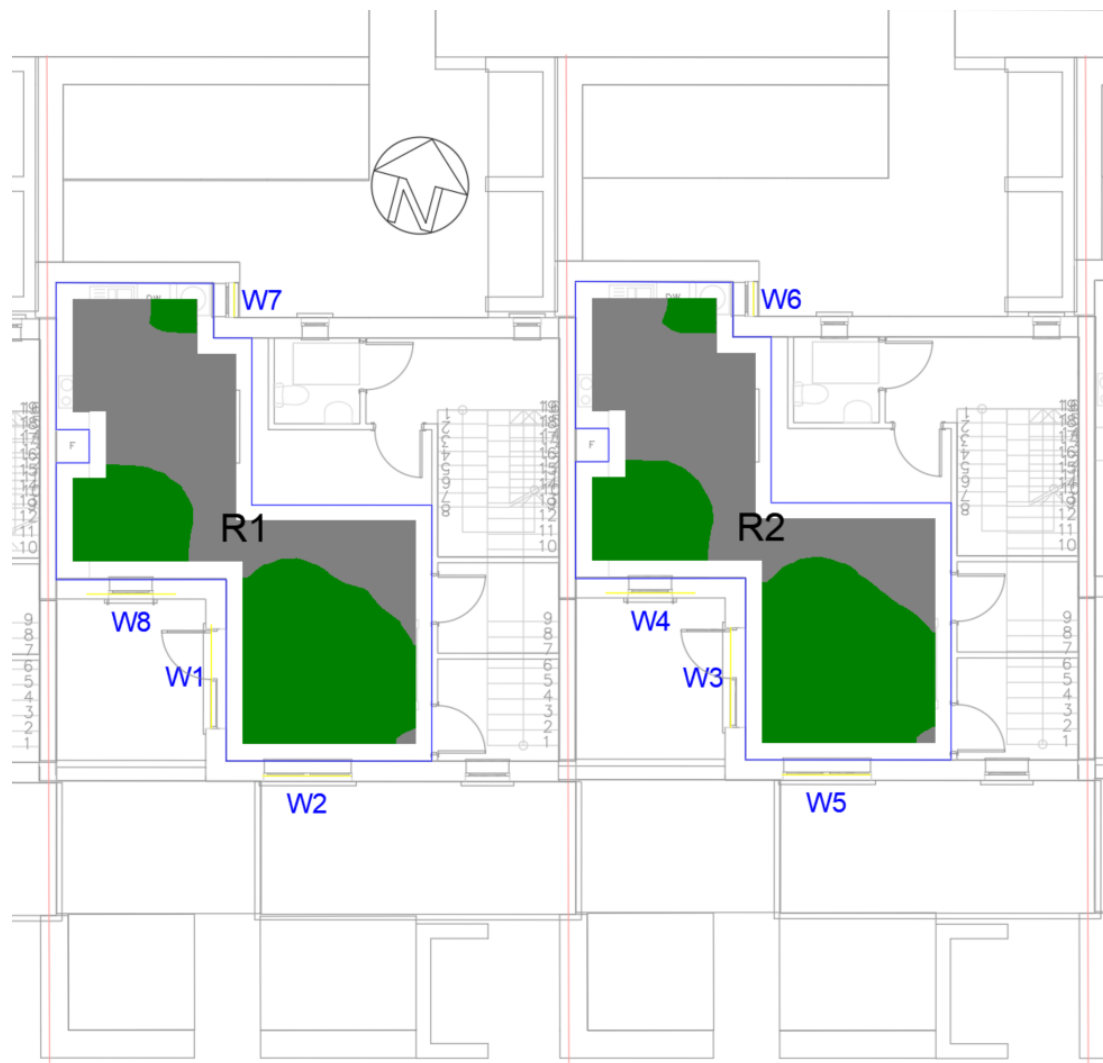
Figure 31: DP-05-06 First Floor sDA Contours
